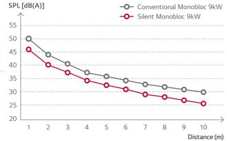
\* Based on 9kW model with low noise mode.
