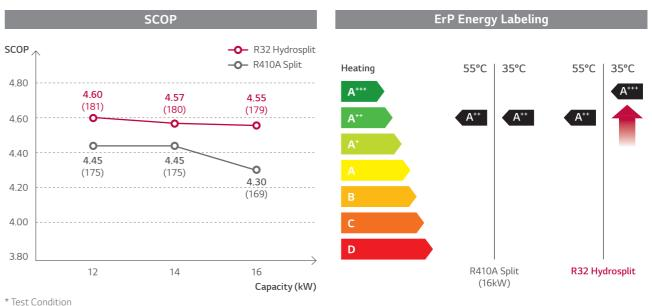
Test procedure follows EN14825 (low temp. average). based on the single phase model line-up.
